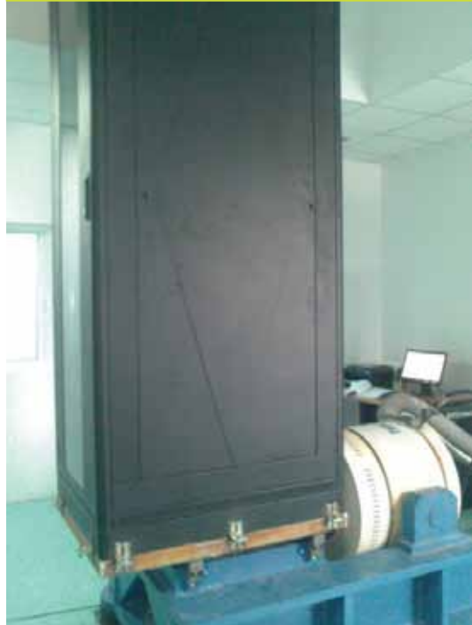
Dinamik yük, titreşim ve mekanik darbe deneyleri (DL4) Dynamic load, vibration and mechanical impact tests (DL4)
